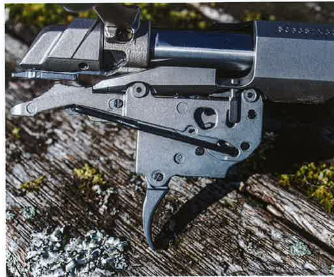
ABOVE & LEFT: The crisp-breaking X-Bolt trigger is user adjustable and easily tuned to suit the individual shooter.
